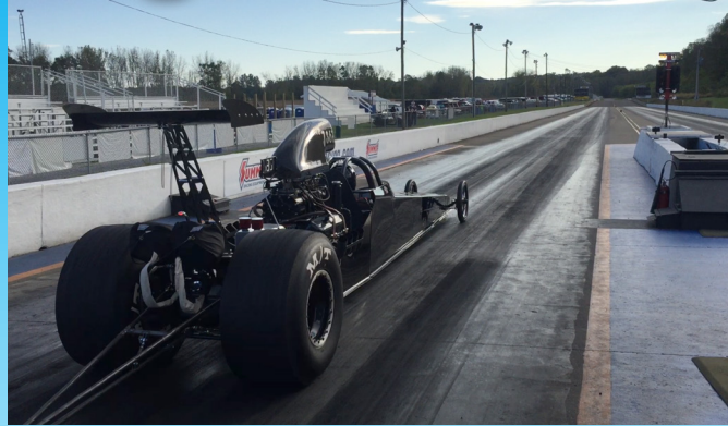
Chassis: 2014 Diamond Race Cars Dragster Motor: Rolla Competition Engines 540 BBC with 14/71 blower.
